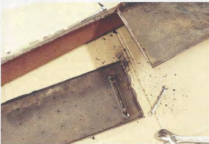
Unlike Ford's 1931 passenger-car line, the pickups, and other commercial vehicles, utilized two-piece splash aprons and all-steel running boards, which are in the process of being separated from each other and the fenders in this image.
