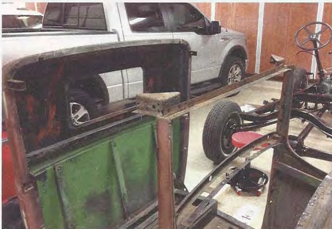
The remaining wooden roof structure appeared to be sound; however, after consulting knowledgeable Model A enthusiasts, it was recommended that all the wood within the cab be replaced with new pieces. Fortunately, dry rot had not affected the steel supports.
